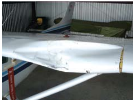
▲ Wing damage from buzzard strike
